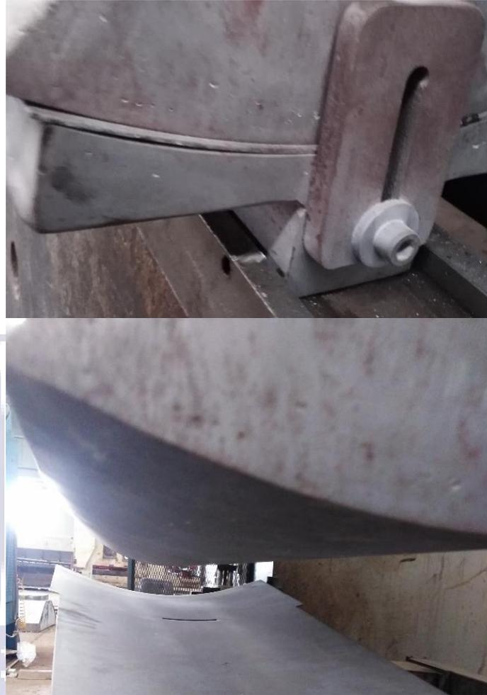
Figure 21. Sails curving die installed on the bending machine during manufacturing the prototypes.
