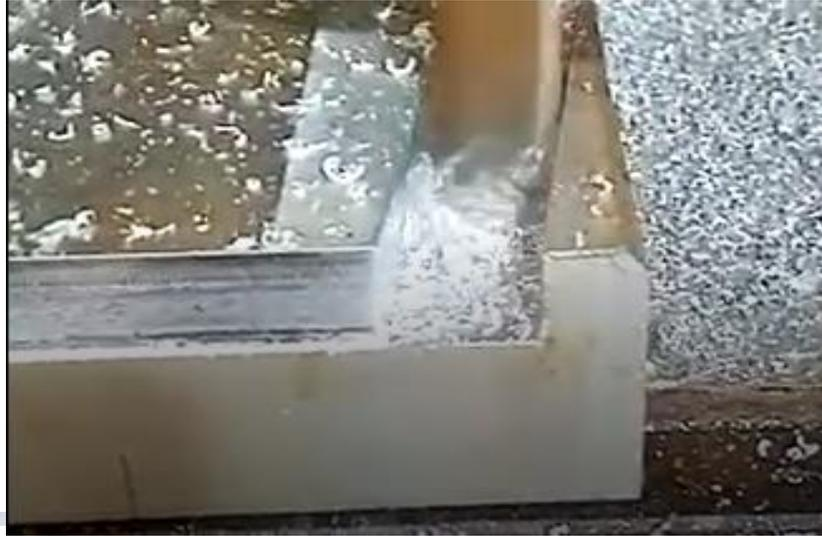
Figure 19. "Z-level" operation of lower Sail die.
