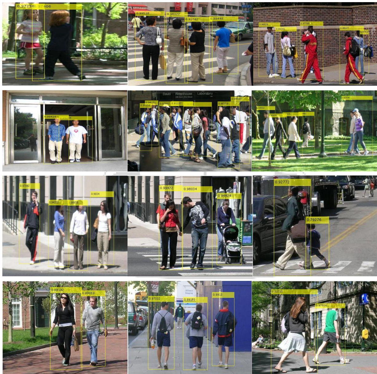
Fig.5: Some experiment results of pedestrian detection on the Penn-Fudan pedestrian Dataset using the Faster R-CNN system. The model is VGG-19 Each output box is associated with a softmax score in [0; 1] . A score threshold of 0.7 is used to display these images.
