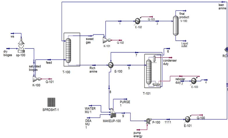
Figure 2.1 Describes the amine absorption process
