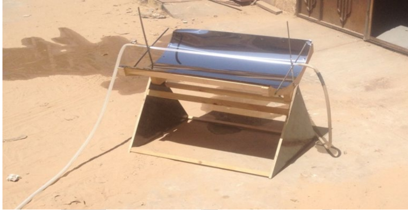
Figure (7) Collector test with a garden hose
