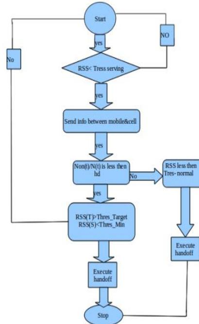
Fig. 2, adaptive algorithm
