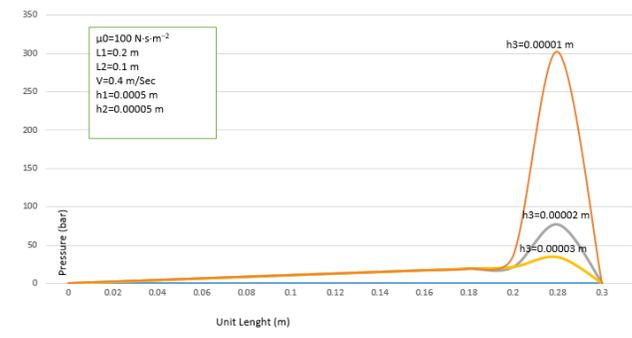
Fig. 3, effect of outlet gap ( $h_3$ ) on pressure distribution within the unit
