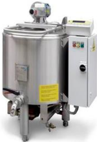
Fig. 1. Pasteurizing milk heat exchanger
