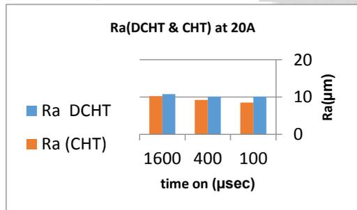
Fig(3c)the variation of surface roughness in CHT process compared with DCHT at 20A
