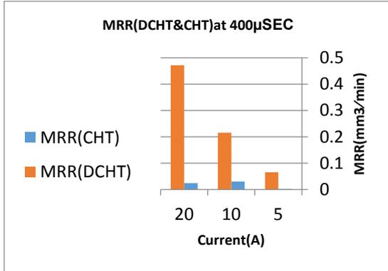
Fig. (6b) the variation of Material removal Rate in CHT process compared with DCHT at 400 µsec.
