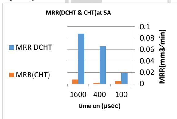
Fig. (5a) the variation of Material removal Rate in CHT process compared with DCHT at 5A.
