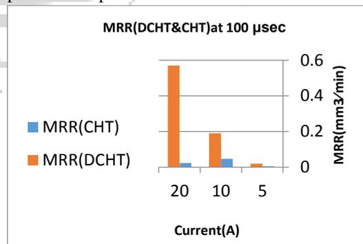
Fig. (6a) the variation of Material removal Rate in CHT process compared with DCHT at 100  $\mu$ sec.
