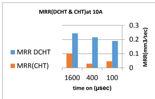
Fig. (5b) the variation of Material removal Rate in CHT process compared with DCHT at 10A.
