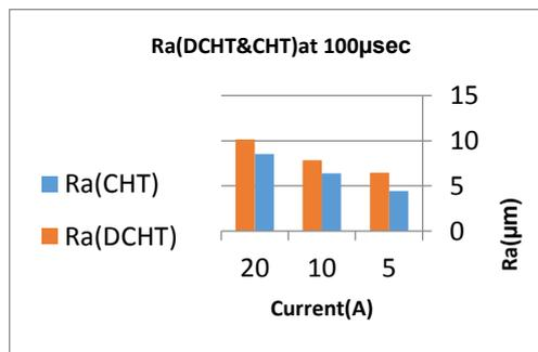
Fig.(4a) the variation of surface roughness in CHT process compared with DCHT at 100  $\mu$ sec
