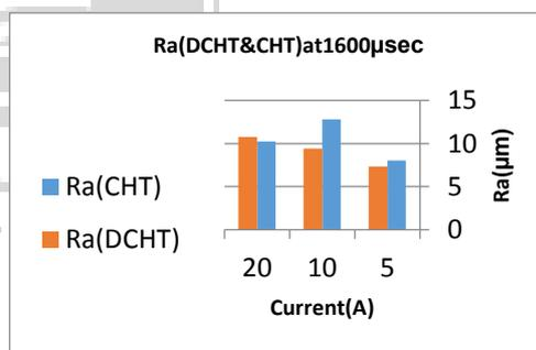
Fig. (4c) the variation of surface roughness in CHT process compared with DCHT at 1600  $\mu$ sec
