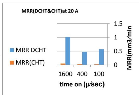
Fig. (5c) the variation of Material removal Rate in CHT process compared with DCHT at 20A.
