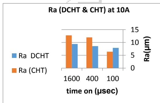
Fig(3b)the variation of surface roughness in CHT process compared with DCHT at 10A.
