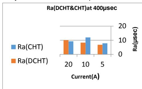
Fig. (4b) the variation of surface roughness in CHT process compared with DCHT at 400  $\mu$ sec.
