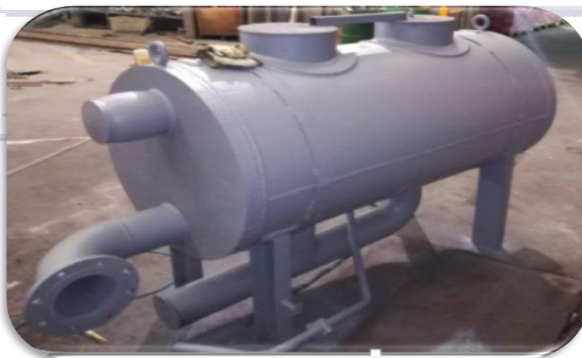
FIGURE No (11) - Repainting evaporator case
