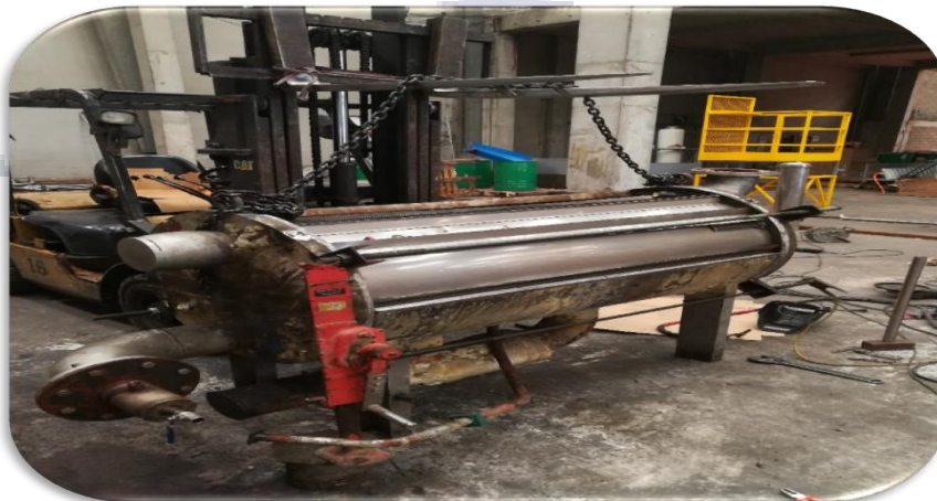
FIGURE No (7)- Placing exchanger its case
