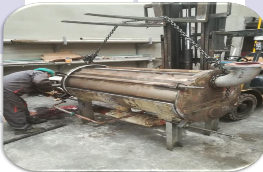
FIGURE No (3) - Reinstalling the evaporator in its pressure case
