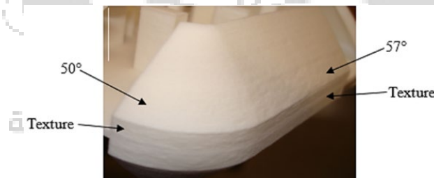
Figure 5: The Characteristic "Orange Peel" Surface Texture Visible on Angled Surfaces (Aged PA2200 Powder).
